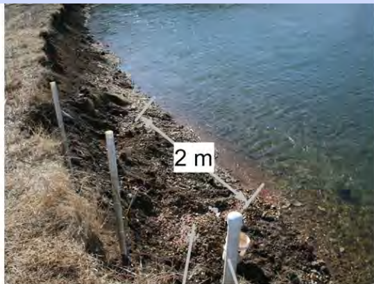
Streambank Seep Emerging from Bank and Entering the Barren Fork Creek
