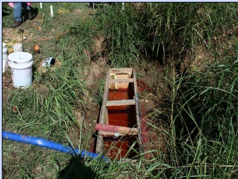
Rhodamine injection into trench
