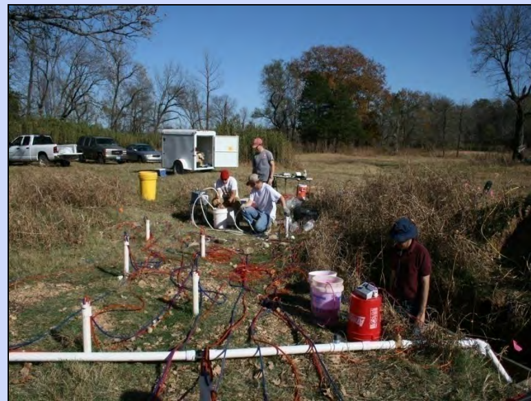
Observation well sampling during tracer/P injection
