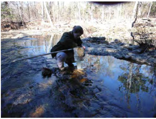
Macroinvertebrate sampling with d-frame dip net
