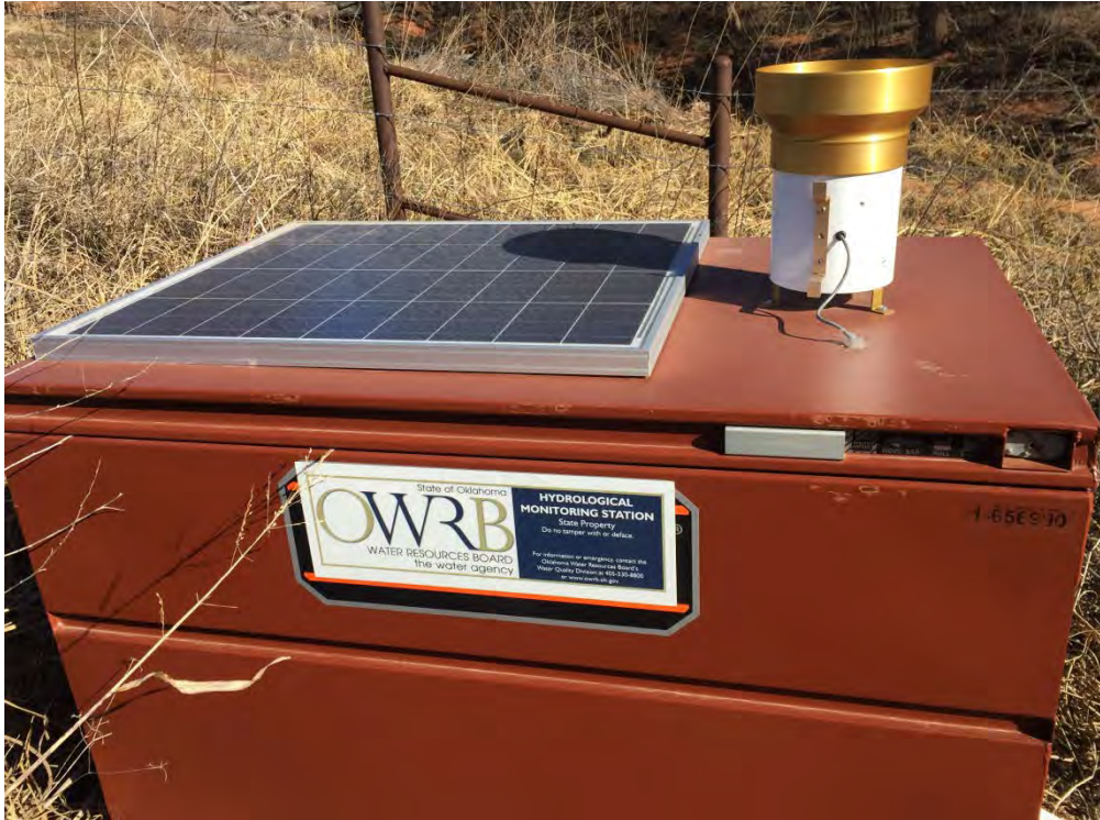
JOBOX® housing the autosampler
